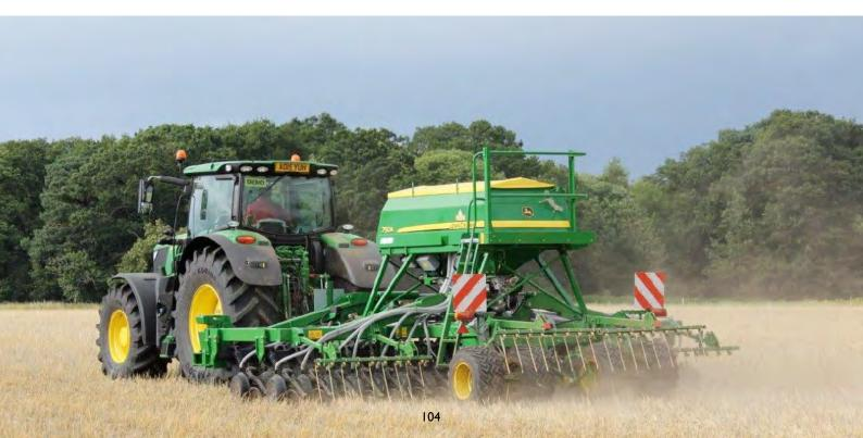
Weaving's introduction to zero-till crop establishment began over 20 years ago and has adapted to meet the demands of the UK farm. With continuous refinements and futureproofing since, Weaving has now developed the GD coulter, a disc coulter design which satisfies all drilling systems. The GD coulter provides remarkably low soil disturbance, has a
